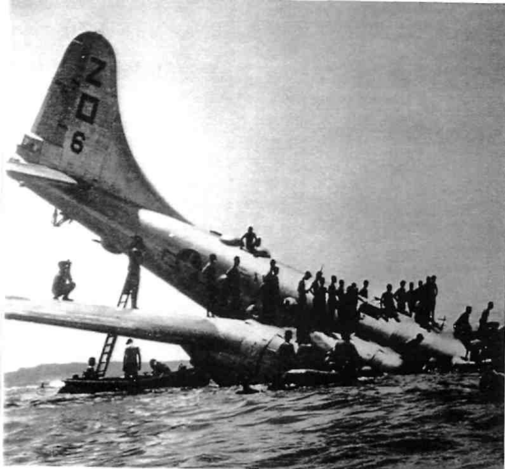
Boeing B-29 Superfortress, "Draggin Lady," lost on February 23, 1945, off the Island of Saipan, Marianas Group. Three lives were lost. The cause of the crash was multiple engine failures. This photograph has been on display in the Smithsonian Institution's National Air And Space Museum in Washington, D.C.
