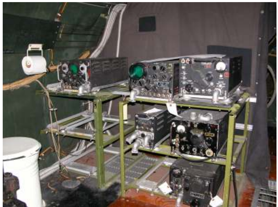
Top: An early countermeasures fit in a standard B-29. (Mike Hanz)
