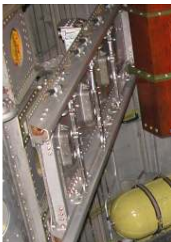
Above: The A-2 Bomb Arming Control.. Diagram from the Bombardier's Information File ( Mike Voisin )
